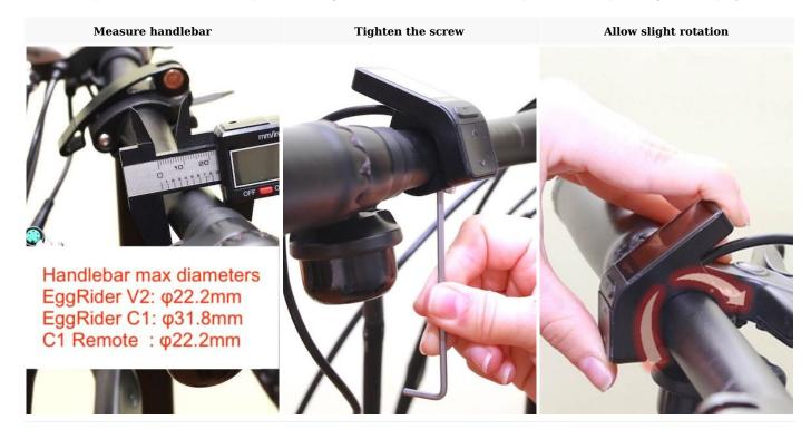
**EggRider V2** is designed for handlebars with a diameter of 22.2mm, and it should be mounted on a straight section of the handlebar.
